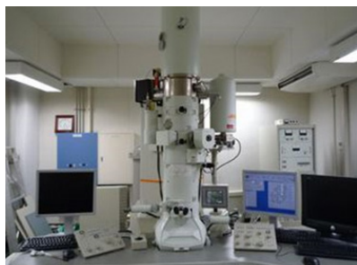
透過型電子顕微鏡 JEM-2100XS
