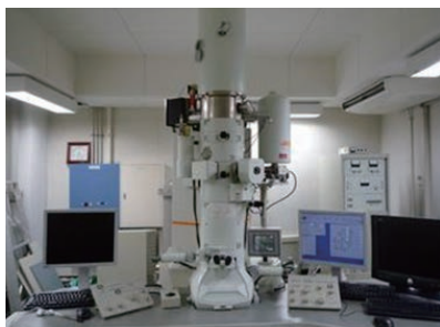
透過型電子顕微鏡 JEM-2100XS
